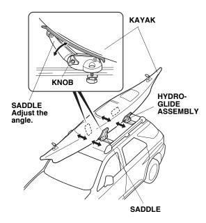
5. Slide the kayak forward or backward until it's level with the roof. If necessary, loosen the knob on each saddle and adjust the saddle angle to fit snugly against the kayak. Tighten each knob securely.
