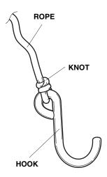
With the hook facing in the direction shown, route the other end of the rope through the bottom of a ratchet.
