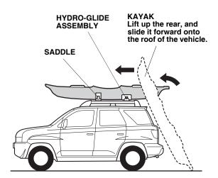
4. Adjust the distance between the saddles and the hydro-glide assemblies to the same width as the kayak, then secure the saddles and the hydro-glide assemblies by tightening the knobs you installed in steps 1 and 2.
