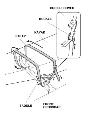
Route the strap under the rear crossbar and around the kayak as shown. Slide the buckle cover away from the buckle, route the strap thru the buckle, and tighten the strap. Slide the buckle cover back over the buckle.
