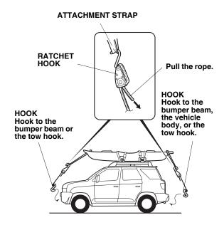
13. To loosen the rope, push up on the ratchet release lever, then pull on the rope.
