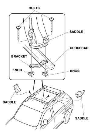
Position the two hydro-glide assemblies on the rear crossbar. Loosely install the hydro-glide assemblies using one bracket, two bolts, and two knobs for each assembly. The distance between the two assemblies should be the same width as the kayak.
