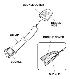
Route the strap under the front crossbar and around the kayak as shown. Slide the buckle cover away from the buckle, route the strap through the buckle, and tighten the strap. Slide the buckle cover back over the buckle.
